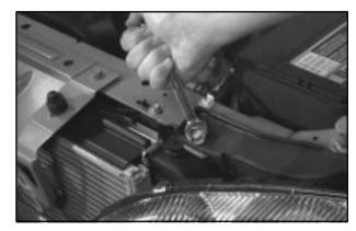
2. Remove the other bolt that anchors the headlamp assembly. Pull the headlamp assembly toward the front of the vehicle to access the bulb assembly.
